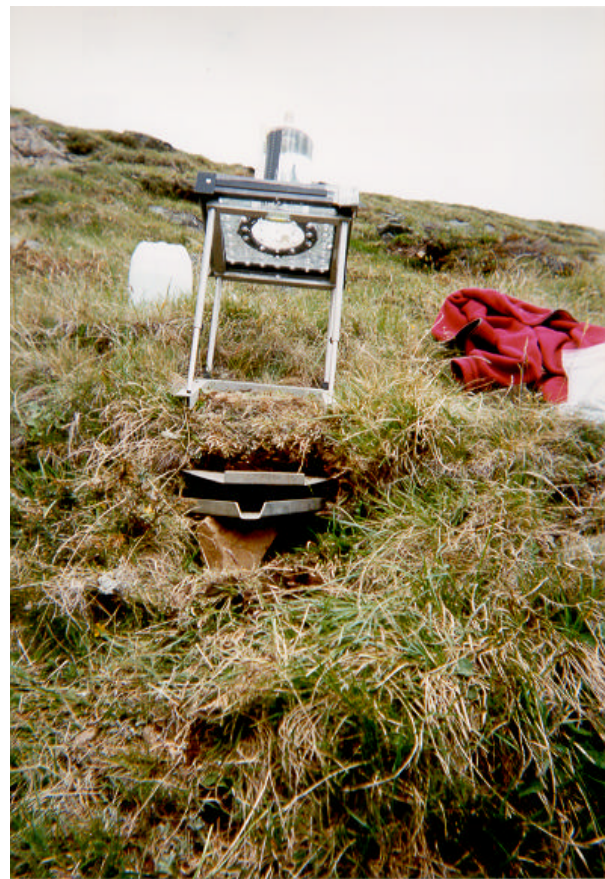
Figure 3.3. The rainfall simulator on a natural slope (rs23).
