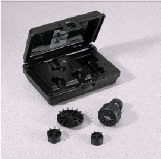
Figure 3.9. A Torvane. A comparable apparatus was used during fieldwork. Source: ELE (2000, p. 80).
