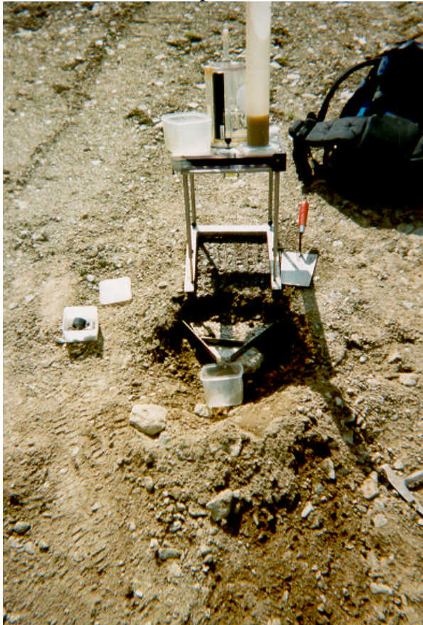
Figure 3.2. The rainfall simulator on a ski piste (rs46).
