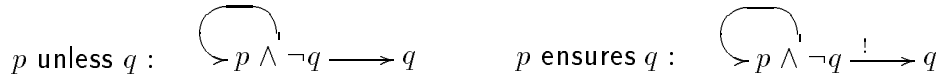
Figure 4.2: unless and ensures. The predicates p \wedge \neg q and q define sets of states. The arrows depict possible transitions between the two sets of states. The arrow marked with ! is a guaranteed transition.
