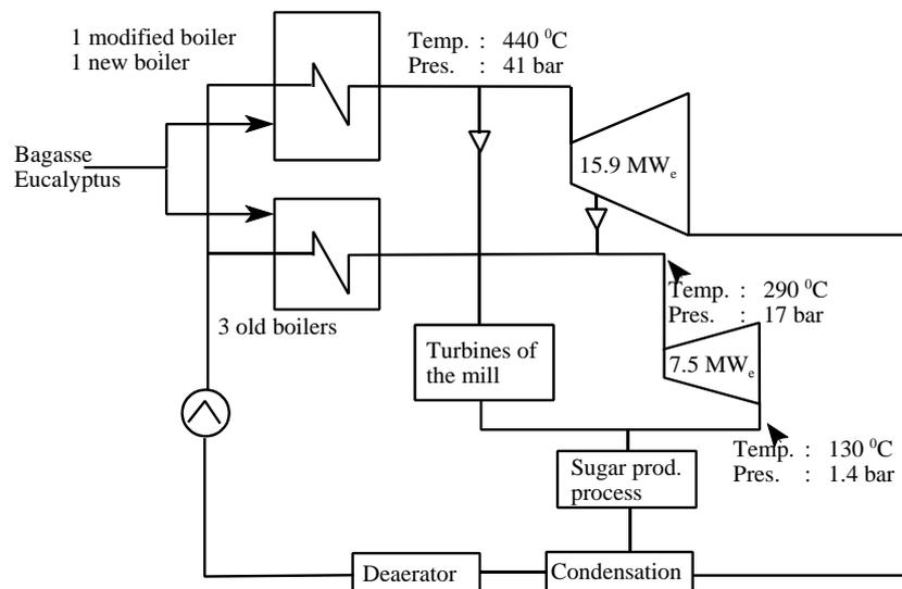
Figure 2. Design of the power plant after extensions at San Antonio. During the sugar season this whole system is used. Outside this season, eucalyptus will be fired only using the full capacity (without steam extraction) of the upper turbine.
