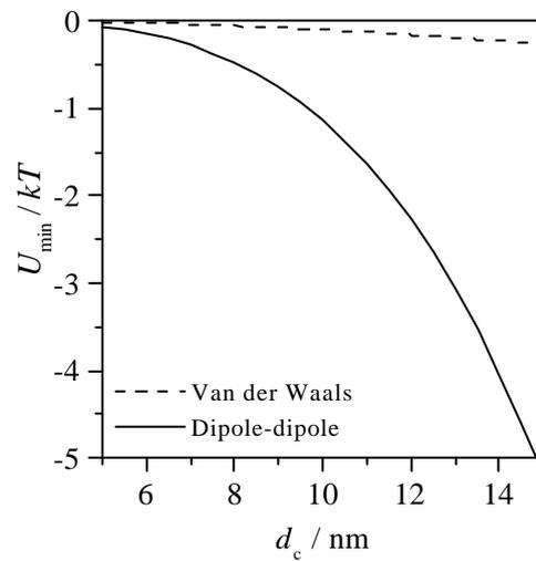
**Figure 3.3.** Size-dependence of Van der Waals and maximum dipole-dipole interaction between two touching magnetic particles.  $d_c$  is the diameter of the  $\text{Fe}_3\text{O}_4$  core. The thickness of the oleic acid layer is taken 2 nm.
