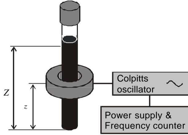
**Figure 5.1.** Schematic drawing of the susceptibility meter setup.
