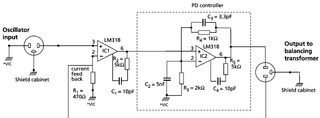
Figure 5.17. Electronic circuit diagram of the transconductance (V-I) amplifier.
