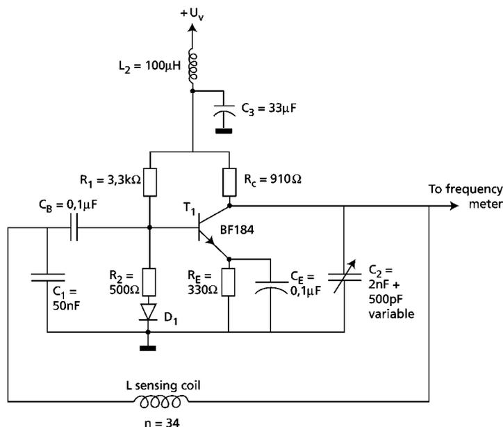
Figure 5.15. Electronic circuit diagram of the Colpitts oscillator.
