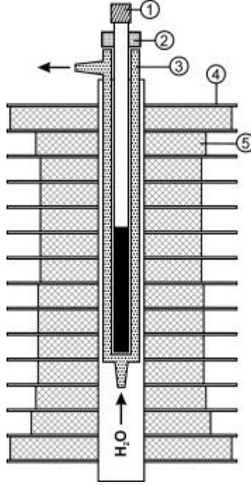
**Figure 6.1.** Schematic drawing of the setup used for phase separation experiments. (1):sample tube; (2):magnetic sensing coil; (3):water-cooled thermostat; (4):copper cooling plates; (5):copper windings
