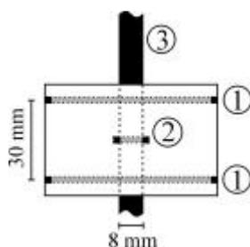
**Figure 3.4.** Schematic drawing of mutual induction coils. 1: Helmholtz coils, generating a homogeneous magnetic field of  $100 \text{ Am}^{-1}$ ; 2: secondary coil, measuring  $c_i$ ; 3: sample tube. The susceptibility meter consists of a measuring coil and a compensation coil, both of the type shown here.
