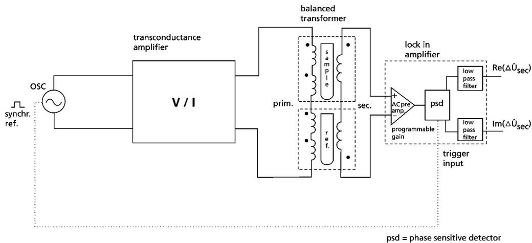
Figure 5.16. Schematic drawing of frequency-dependent complex susceptibility meter.
