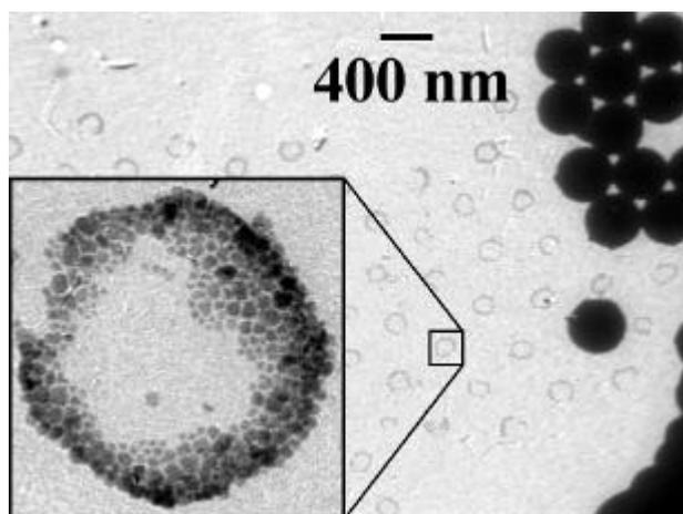
**Figure 7.2.** TEM picture of a grid with coated silica spheres. Some silica spheres have been removed by gentle wiping with tissue paper, making rings of magnetite particles visible (enlargement) that had accumulated between the silica sphere and the grid.
