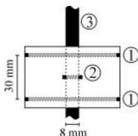
**Figure 5.18.** Schematic drawing of one of the branches of the balanced transformer. The susceptibility meter consists of a sample branch and a reference branch, both of the type shown here. 1: Helmholtz coils, generating a homogeneous magnetic field of  $100 \text{ Am}^{-1}$ ; 2: secondary coil, measuring  $\chi$ ; 3: sample tube.
