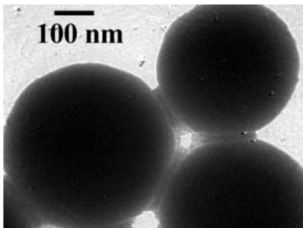
**Figure 7.1.** TEM picture of silica spheres coated with magnetite particles. The coating is accumulated in the most narrow spaces, whereas the rest of the silica surface contains almost no magnetite.
