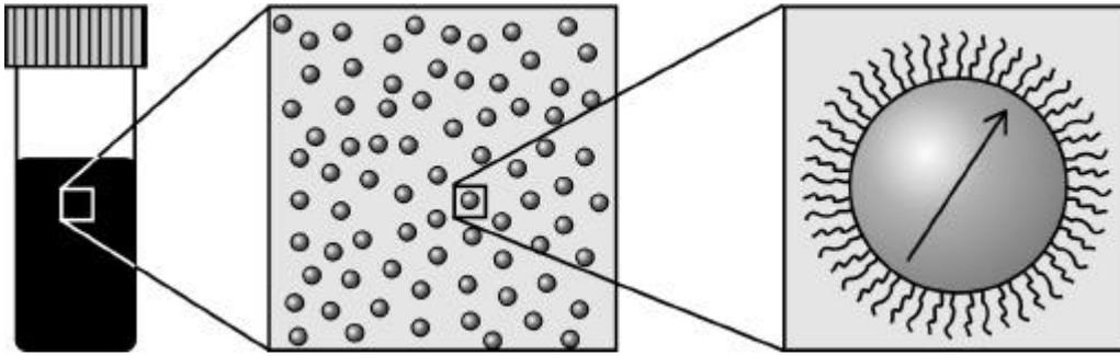
**Figure 1.3.** Schematic drawing of a ferrofluid on three length scales. On the macroscopic length scale (left), it resembles an ordinary liquid. On the colloidal length scale (middle), the fluid appears to consist of small solid particles dispersed in a liquid. Each particle consists of a single domain magnetic iron oxide core, and a surface grafted with polymer chains (right).
