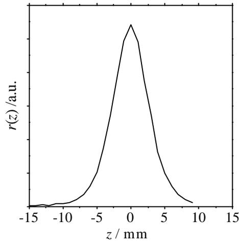
**Figure 5.2.** Measured response function of the sensing coil.
