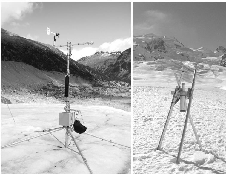
Figure 1.8: Left: automatic weather station on the tongue of Morteratschgletscher. Right: sonic height ranger, about 40 cm above the glacier surface.
