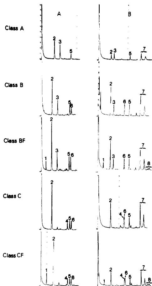
FIGURE 1: Gas-liquid chromatograms of methylated methylglycosides before (A) and after (B) peracetylation. The designations of the peaks (1-8) refer to the following compounds: methyl 2,3,4-tri- O -methylfucoside (peak 1), methyl 2,3,4,6-tetra- O -methylgalactoside (peak 2), methyl 3,4,6-tri- O -methylmannoside (peak 3), methyl 3,4-di- O -methylmannoside (peak 4), methyl 2,4-di- O -methylmannoside (peak 5), methyl 3,6-di- O -methylmannoside (peak 6), methyl 3,6-di- O -methyl- N,N -acetylmethylglucosaminide (peak 7), and methyl 6-mono- O -methyl- N,N -acetylmethylglucosaminide (peak 8).
