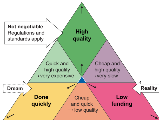
Figure 5: The 'Triangle of Project Management': You can pick only two of the three triangle points, the third one is automatically excluded. Note that developing complex medical devices anyhow requires considerable persistence. For a complex active medical device (such as a kidney replacement device), it typically takes ~10 years to reach market approval, even if all parameters are optimized (depicted by the blue spot in the middle).
