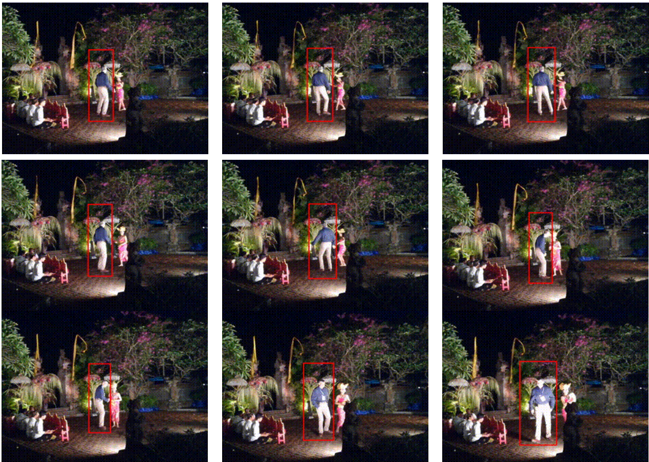
Figure 10. Tracking a dancing man. Nine frames from the video are provided, with frame order from top to bottom and from left to right. The background is dynamic, with other moving objects in the frame. The ROI is shown in red.
