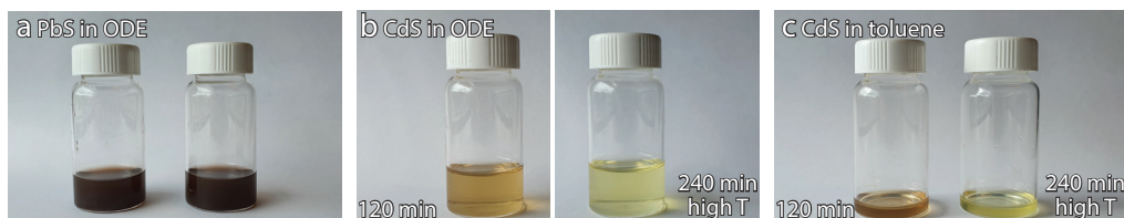
Figure S6.3 Pictures of the PbS NSs before (a) and after cation exchange (b and c). The initially dark brown dispersion turns light brown or orange, or even yellow in case of prolonged reaction times at higher temperatures. After purification, these colors are retained (c).
