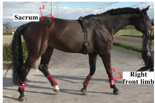
Fig. 1. IMUs locations and orientations on horse body.
