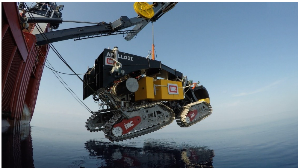
Figure 5.2: Deployment of the Apollo II pre-prototype nodule collector vehicle from the aft of RV Sarmiento de Gamboa during the 2018 field test in Málaga Bight. Photo courtesy: Alberto Serrano. Note the Nortek Aquadopp current profiler mounted upward-facing on starboard side of the diffuser. Acoustic backscatter data presented in Fig. 5.11E were acquired with the current profiler mounted backward-facing.
