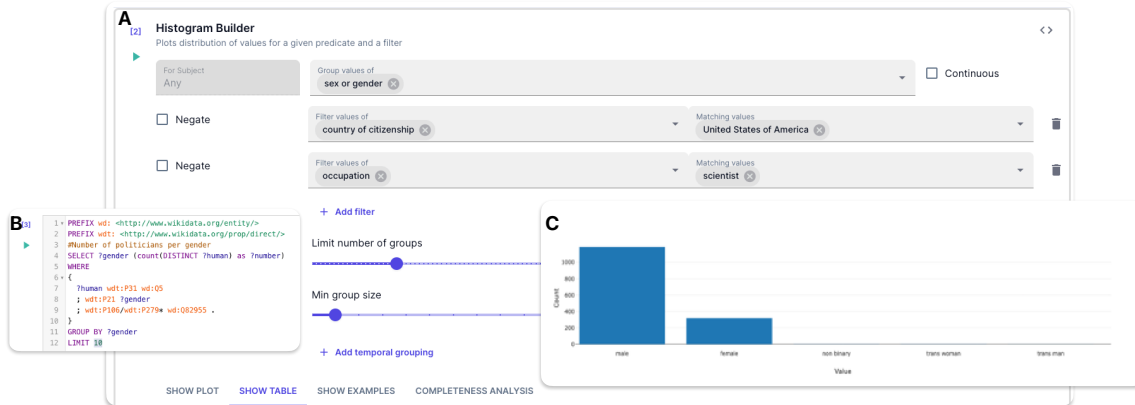
Figure 3: A) Widget that is used to generate the barplot in (C) when run on Wikidata. B) A query to accomplish the same.
