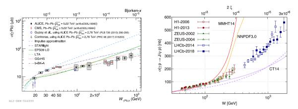
Fig. 2  $J/\psi$  photoproduction cross sections for  $\gamma$ Pb (left) from ALICE [49] and CMS [50] measured using nuclear breakup categories to unambiguously determine the energy dependence and for  $\gamma$ p (right) from HERA and LHCb measurements versus NLO predictions [57]
