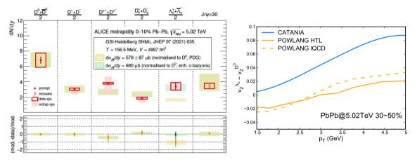
Fig. 8 Left: charm hadron yields in central PbPb collisions, data [14] and SHM predictions. Note the scale factor of 30 for the  $J/\psi$  meson. Right: The difference between the  $v_2$  values of  $\Lambda_c^+$  and  $D^0$  as a function of  $p_T$  as predicted by the Catania coalescence model and POWLANG
