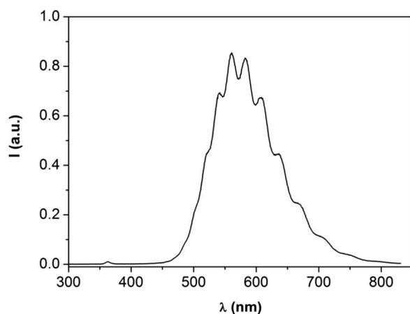
**Figure 2.** EL spectrum of n-type GaN recorded in a 0.1 M  $S_2O_8^{2-}$  solution of pH 13.
