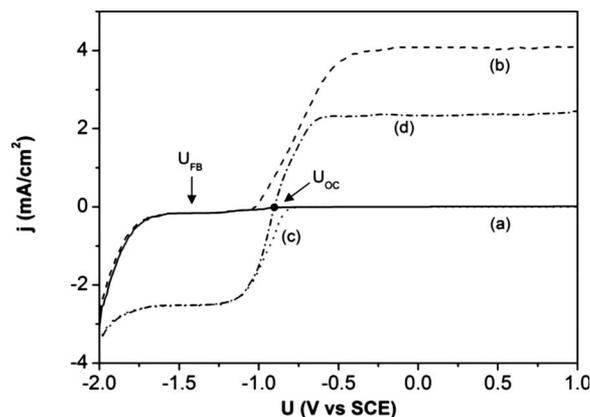
**Figure 1.** Current density–potential plots for n-type GaN in a 0.02M KOH solution recorded (a) in the dark and (b) under illumination. After addition of 0.02 M  $S_2O_8^{2-}$ , curve (c) is obtained in the dark, and curve (d) is obtained under illumination. The potential was scanned at a rate of 10 mV/s. The solution was not stirred.  $U_{FB}$  is the flatband potential of GaN in KOH solution.
