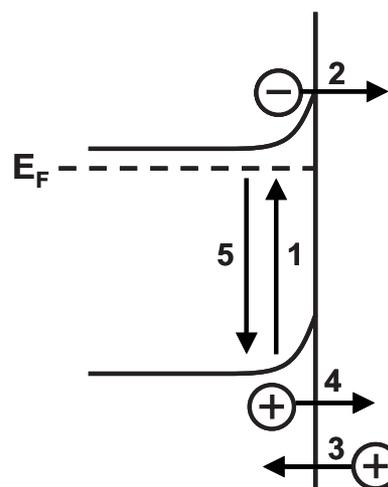
**Figure 3.** Schematic representation of the steps occurring during electroless photoetching of n-type GaN in a KOH/ $S_2O_8^{2-}$  solution.  $E_F$  indicates the Fermi level of the semiconductor.
