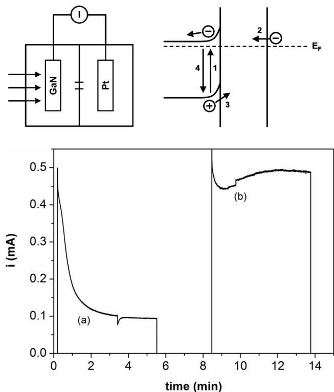
**Figure 4.** Schematic representation of a two-compartment photogalvanic cell and the corresponding band-energy diagram (top). (a) The photocurrent-time plot was recorded with 0.02 M KOH solution in both compartments. (b) When 0.02 M  $S_2O_8^{2-}$  was added to the compartment of the Pt counter electrode, the photocurrent density increased.
