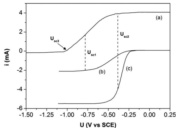
**Figure 5.** (a) Current-potential plot for photoanodic dissolution of GaN in a 0.02 M KOH solution. (b) Corresponding plot for reduction of  $S_2O_8^{2-}$  at a Pt electrode in a 0.02 M KOH/0.02 M  $S_2O_8^{2-}$  solution. (c) When the surface area of the Pt is increased, the reduction current increases. The photoanodic curve is corrected for absorption by  $S_2O_8^{2-}$ .
