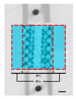
**Figure 1.** Region of interest on micro-CT scanning. Bone volume inside (BVi) and bone volume outside (BVo) are defined as bone formed inside and outside the porous space and the medullary canal of the titanium implants. Scale bar indicates 1 µm.
