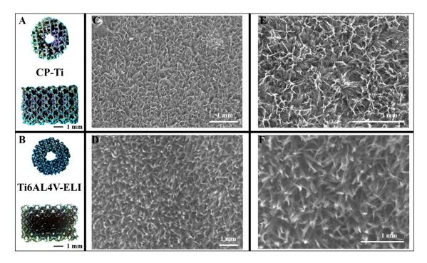
**Figure 2.** SEM images of CP-Ti and Ti6Al4V ELI porous implants. Macroscopic overview (**A**,**B**), and enlarged details (**C**–**F**) of the two different porous titanium implants. Panels (**E**,**F**) are zoomed in pictures of panels (**C**,**D**).
