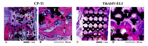
**Figure 5.** Histological evaluation of bone bridging. Representative transversal sections of femur defects eleven weeks after implantation of porous titanium implants; CP-Ti (**A**) and Ti6Al4V-ELI (**C**), including detailed view for CP-Ti (**B**) and Ti6Al4V-ELI (**D**). Sections are stained with basic fuchsine and methylene blue. Basic fuchsine stains bone pink, methylene blue stains fibrous tissue blue. B = bone, BM = bone marrow, F = fibrous tissue, T = titanium.
