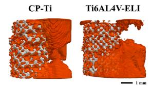
**Figure 7.** Illustration of bone bridging. Representative 3D micro-CT images showing the average extend of bone bridging of the CP-Ti and the Ti6Al4V-ELI titanium implants.
