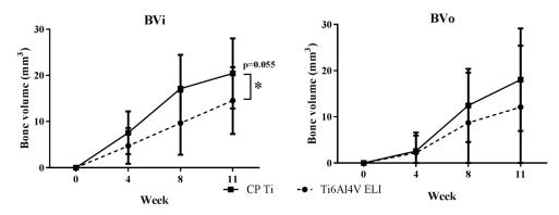
**Figure 3.** Longitudinal quantification of bone regeneration. In vivo  $\mu$ CT scans after zero, four, eight, and eleven weeks; BVi and BVo: defined as bone formed inside and outside the porous space and in the medullary canal of the titanium implants. Values are expressed as mean and SD (n = 8 for CP-Ti and n = 8 for Ti6Al4V-ELI). \* Indicates (borderline) significant differences between groups.
