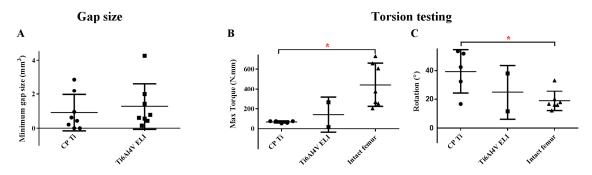
**Figure 6.** Bone bridging and mechanical strength. The remaining gap size after eleven weeks was used to indicate bridging success (**A**). Mechanical femoral strength (**B**) and rotation (**C**) after implantation of different types of porous titanium implants measured by torsion tests. \* indicates significant differences between groups.
