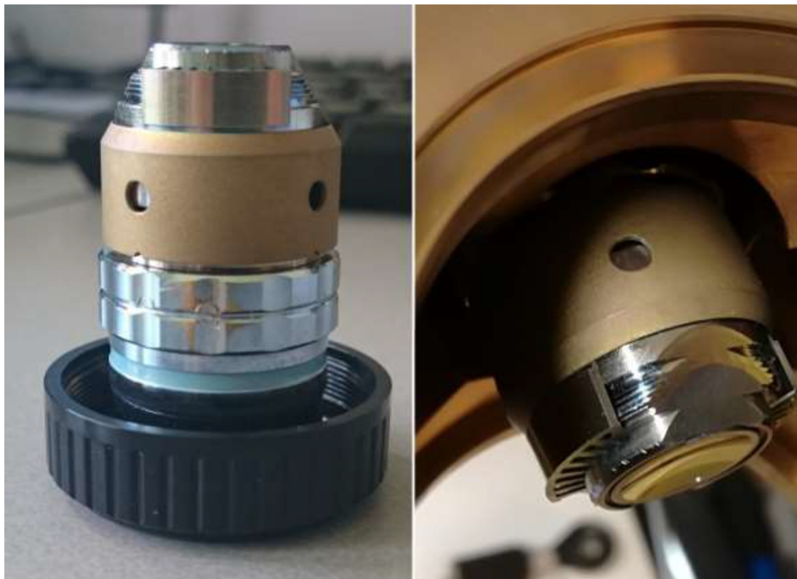
Fig. 3. Photographs showing the objective. Part of the objective is milled away to make it fit close enough to the specimen. The right photograph shows the objective mounted on a TEM octagon.
