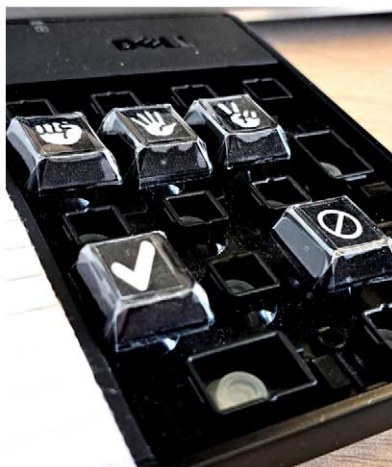
Fig. 5. Tailored control pad used in the second design to interact with the robot.
