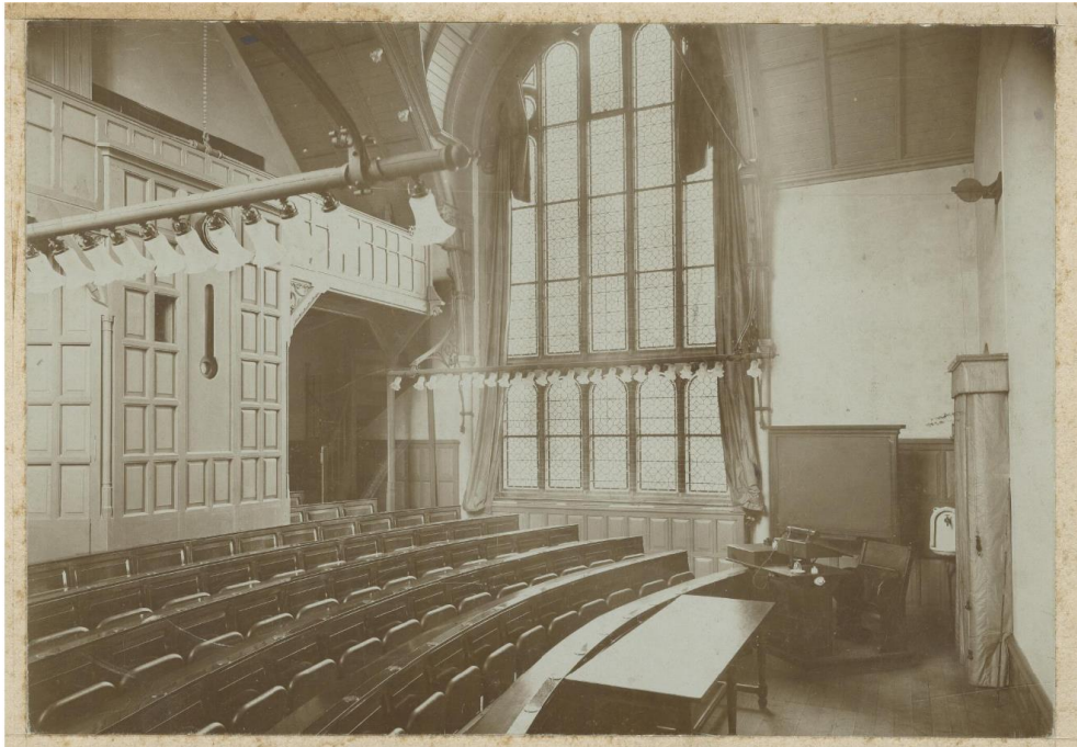
Figure 12. Lecture hall at the Botanical Laboratory in Groningen. The entire arrangement is determined by the use of the optical lantern; projection room at the back, lighting system to enable notetaking, placement of the lectern, seating arrangements. (Beeldbank Groningen (Image database Groningen)). 138
