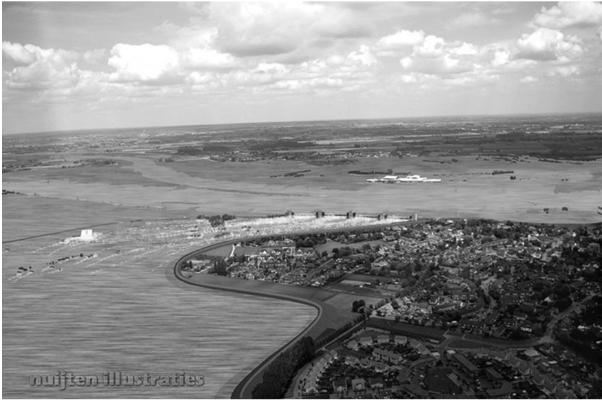
FIGURE 3.1 Illustration of the inlet of the proposed retention area of the village Millingen in the Ooijpolder. At a later stage, the water will flow into the village dike ring, the so-called bathtub effect. Source: Studio Nuijten, Kekerdom
