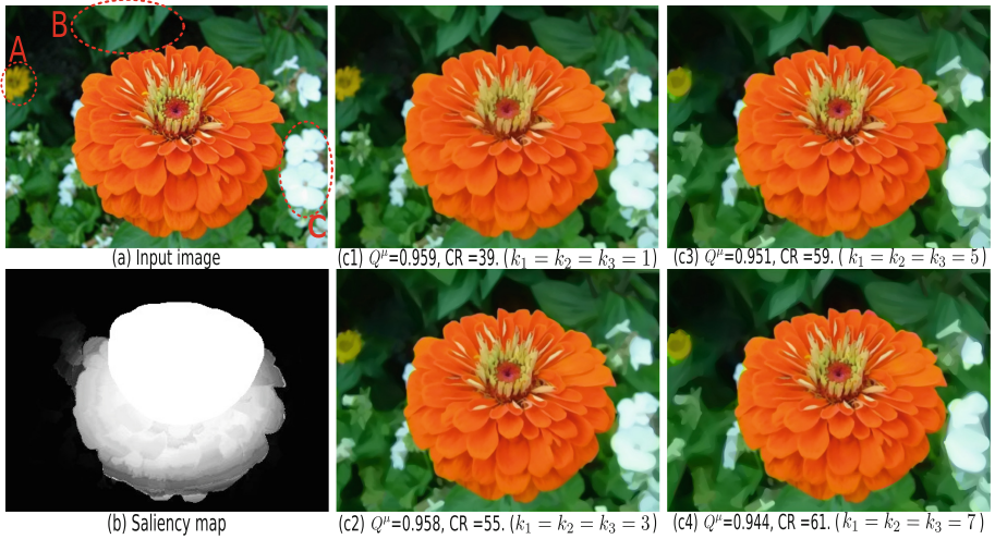
Fig. 9. Progressive simplification of a flower image (a) using a saliency map (b) for different weight values k_1 , k_2 , and k_3 (c1–c4).
