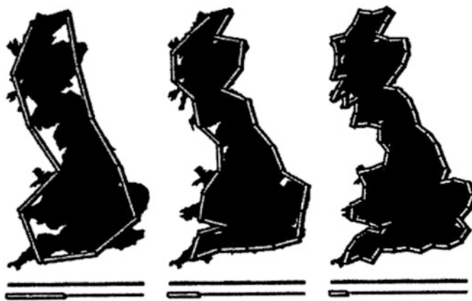
The coast of the United Kingdom is highly sinuous, resulting in divergent estimates of coastline length depending on the unit of measurement. In this image, measurement units of 200 km, 100 km, and 50 km (from left to right) result in length estimates of 2350 km, 2775 km, and 3425 km, respectively. 35
