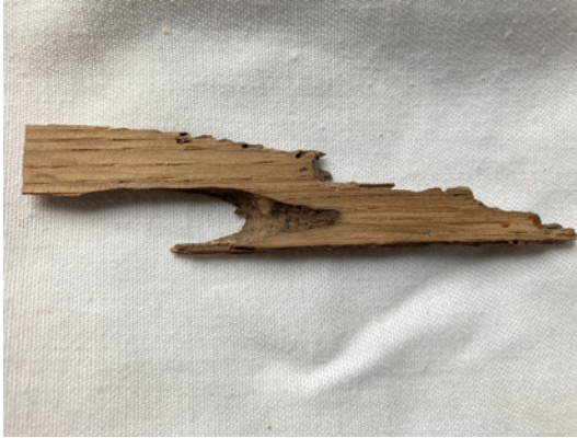
FIGURE 2.15 Oak wood fragment infested with woodworm © MARTA AJMAR
