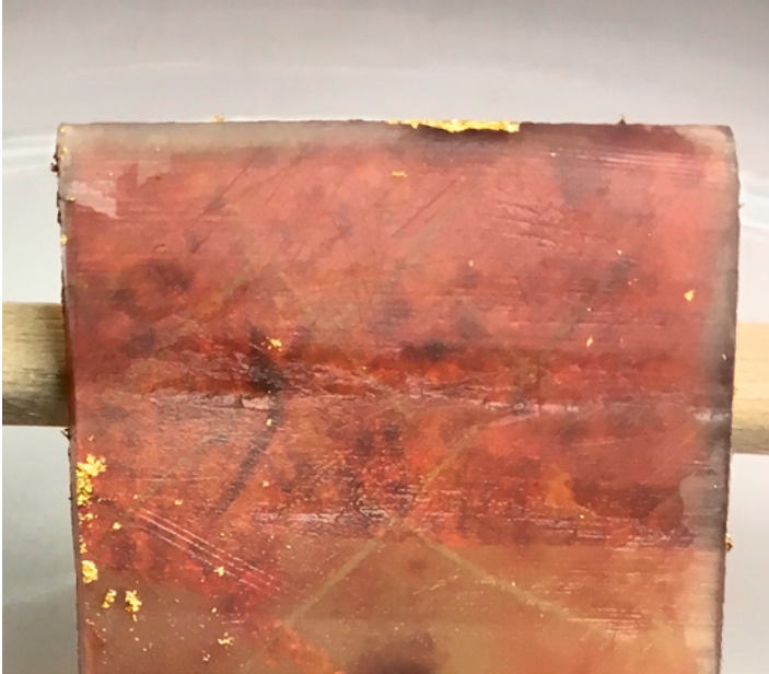
FIGURE 1.4 Imitation jasper from second trial made from bovine horn, red paint (madder and spike lavender varnish), dyed woollen yarn, and transfer gold leaf, oiled with spike lavender oil, following Ms. Fr. 640, fol. 10r
