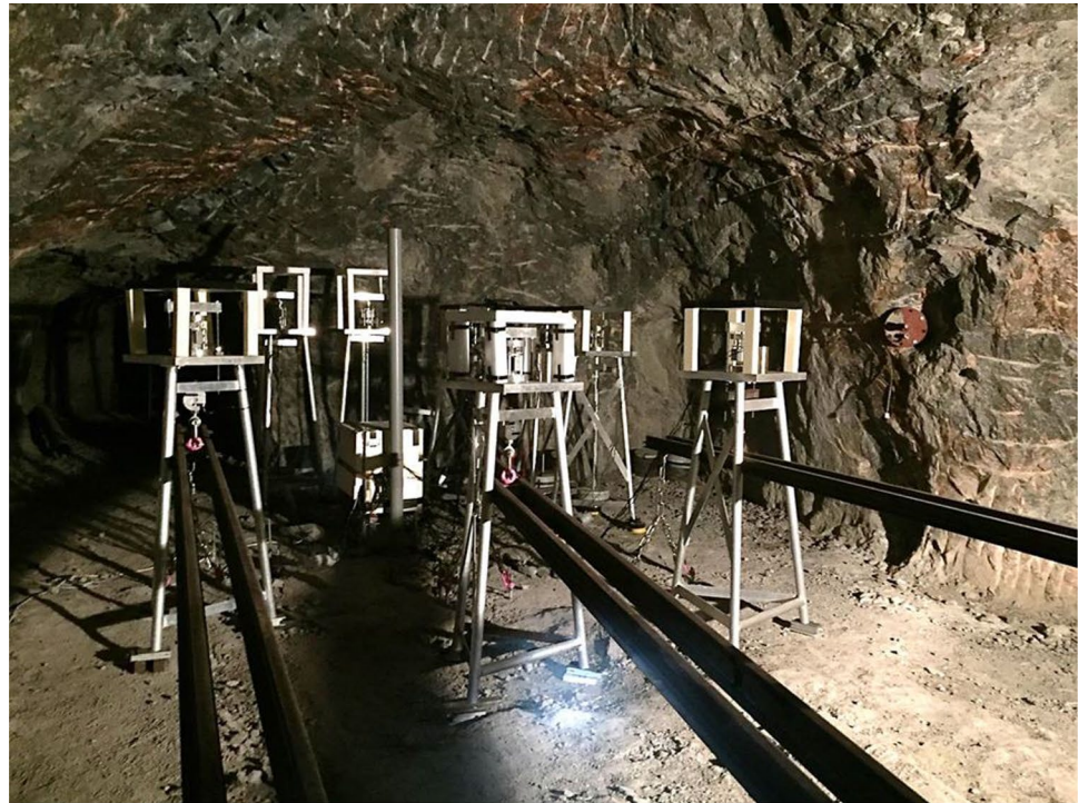
Fig. 3 The three cantilever systems used during the Phase 2 experiments reported here. a Overall view in the mine; b detail of a force-multiplier system and sample
