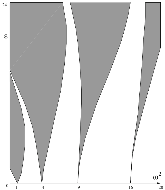
Fig. 3 The gray Floquet tongues denote for which parameter values \omega and \varepsilon the trivial solution of the Mathieu equation is unstable. In our approximations, we have described the lower part ( \varepsilon small) of the tongue emerging from \omega = 1 as in Eq. (2), the tongue shapes for large values of \varepsilon and other values of \omega were obtained numerically
