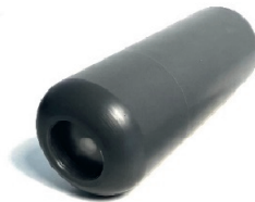
Figure 4. Wireless sensor bolus to measure reticulorumen contractions in a cow.
