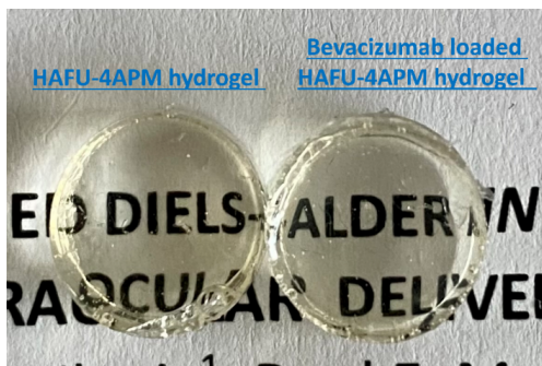
SI-Figure 10 Image of transparent 20 wt% HAFU-4APM hydrogels (diameter 8 mm, 4 mm height) formed at 37 °C with and without loading of bevacizumab.
