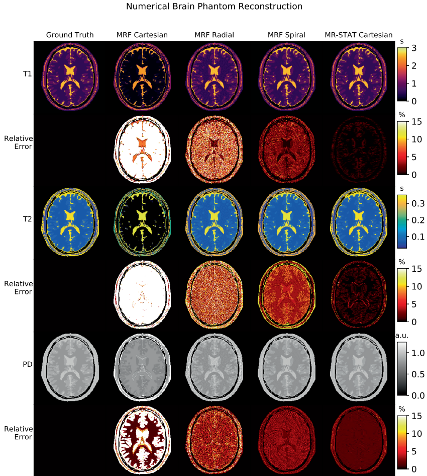
Figure 3.3: [First column] Ground truth T_1 , T_2 and proton density maps for the numerical brain phantom. [Second, third and fourth columns] Reconstructed parameter maps and relative error maps for MRF with linear Cartesian, golden angle radial and golden angle spiral trajectories, respectively. [Fifth column] Reconstructed parameter maps and relative error maps for MR-STAT using a linear, Cartesian sampling trajectory. The MRF spiral and MR-STAT reconstructions both show excellent agreement with the ground truth values. The radial MRF reconstructions show residual aliasing artefacts and the Cartesian MRF reconstruction is heavily biased.
