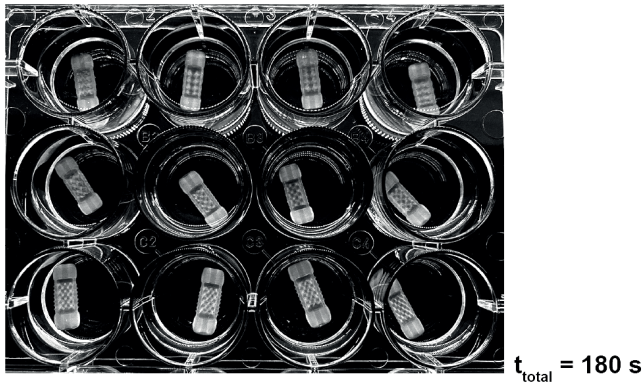
Supplementary Figure S15: High-throughput printing of highly complex, perfusable structures within minutes. Twelve volumetrically printed constructs of complex architectures (Schwarz D, G and P) each measuring 1.7 cm in length and 6 mm in diameter with perfusable inlets printed in 180 s for high-throughput analysis of organoid activity.
