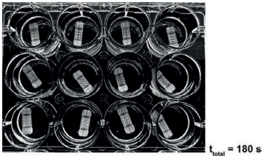
Figure S14. High-throughput printing of highly complex, perfusable structures within minutes. Twelve volumetrically printed constructs of complex architectures (Schwarz D, G and P) each measuring 1.7 cm in length and 6 mm in diameter with perfusable inlets printed in 180 s for high-throughput analysis of organoid activity.
