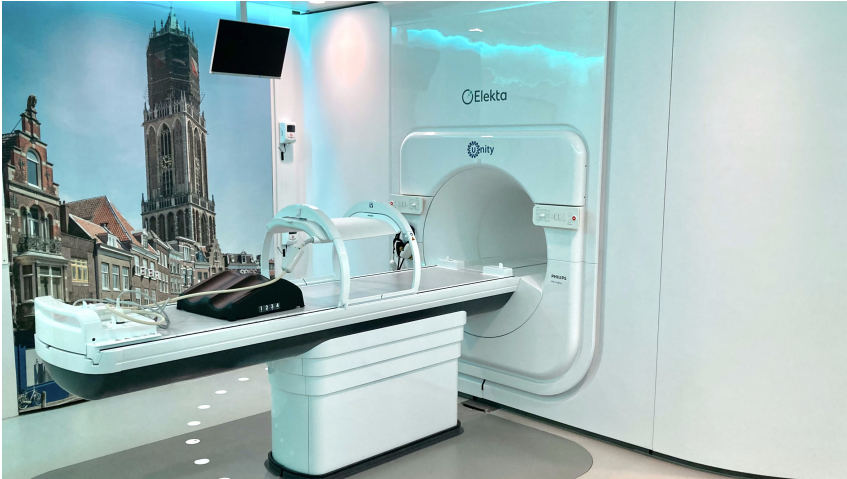
Figure 1.2 Example hybrid MRI/Linac scanner. Hybrid MRI-Linac scanners combine an MRI scanner for image guidance with a linear accelerator for dose delivery. The Elekta Unity is pictured, a commercially-available MR-Linac that combines a 1.5 T MRI with a 7 MV linac.
