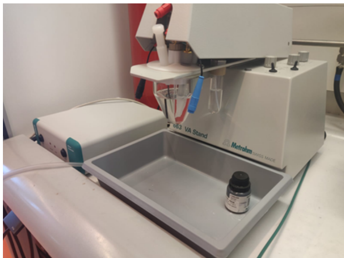
Figure D16. 663 VA stand Metrohm (electrochemical mercury setup).
