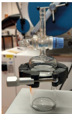
Figure 2.2 Image of a glass-reactor used in the gas-phase ethylene pre-polymerization of the investigated metallocene-based catalyst materials.
