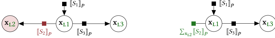
(a) A \vdash_2 -well-typed program with parameters \mathbf{x} . (b) Eliminating \mathbf{x}_{L2} consists of modifying only \llbracket S_2 \rrbracket_p .
