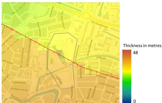
Figure 2.1: Thickness of the Waalre formation at the location of the Griftpark, the fault line is indicated with a red line [79]. The vertical barrier around the Griftpark is indicated by a dark blue line.
