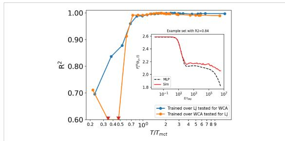
Figure 5. Model transferability of the MLP. We report the  $R^2$  score of the model when tested for a different interaction potential not included in the training. The inset qualitatively shows that  $R^2 > 0.8$  corresponds to acceptable predictions.
