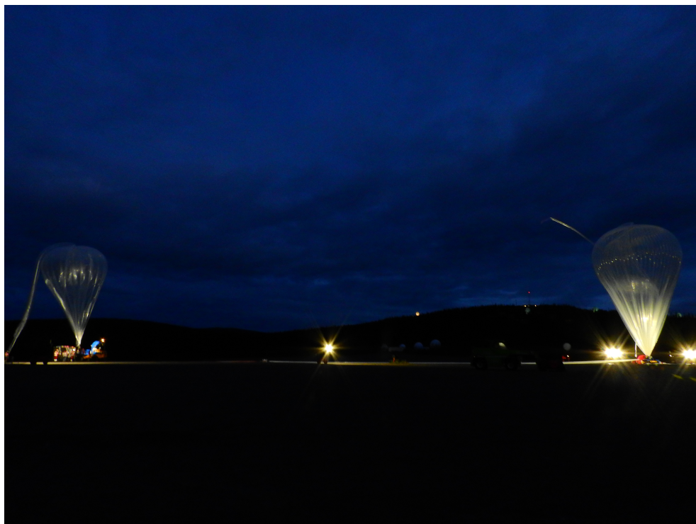
Figure 3.3: The two balloons just before launch during the HEMERA KLIMAT 2021 campaign 2021 at Esrange, Sweden. The left balloon is the auxiliary balloon carrying and stabilizing the TWIN gondola for the very first part of the ascend, before the main, large balloon (right) takes over.
