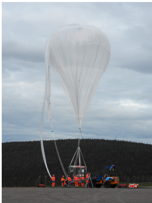
Figure 3.2: Picture of the auxiliary balloon attached to the TWIN gondola during the HEMERA KLIMAT 2021 campaign at Esrange, Sweden.
