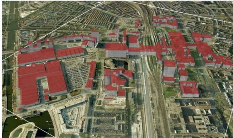
Figure 1: 3D model with level of detail 2 (LOD2) created in CityGML for 2015. This forms the basis for further solar potential analysis.
