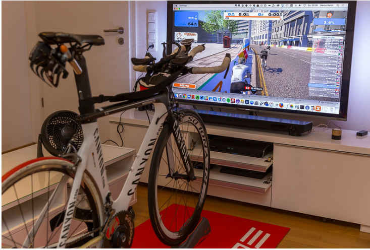
Fig. 1. A typical hardware setting for using Zwift. The bike is placed in a smart trainer which adapts to the route on the screen, thereby offering a resistance in line with the virtual route.
