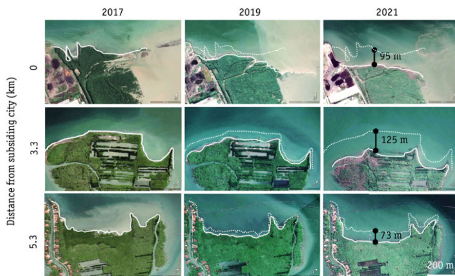
Figure 7-6: Lateral erosion at the three sites closest to the subsidence city.
