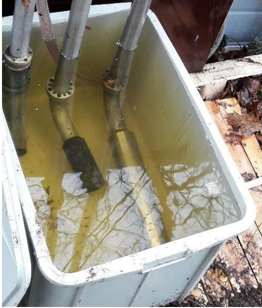
Figure S11 The flow through vessel (open) with, from left to right: Phosphax's auto analyzer intake, and Solitax and Nitratex sensors. The equipment is placed in the hut behind.
