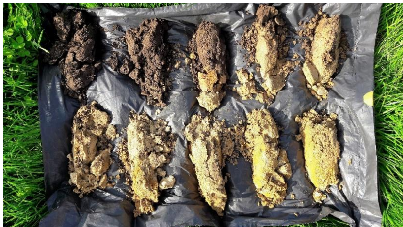
Figure 2-4 On-site picture of soil sample number 19 (0-100 cm). The topsoil was rich in organic matter followed by a horizon which was brown-red-orange colored due to the presence of iron oxides underlain by a gray-yellow to red-orange sand layer
