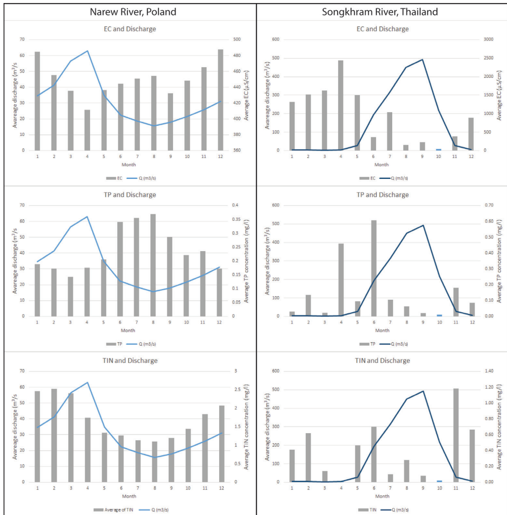
Fig. 5.3 Annual patterns of discharge (lines), EC, TP, and TIN (bars) of the River Narew (St. Gora station) and the River Songkhram (Ban Tha Kok Dang stations). The plots present average monthly values.
