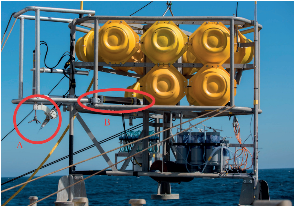
Figure 3.2: The ALBEX lander (Duineveld et al. 2004) equipped with A) the AEC instrument; B) Fluorescence sensor.
