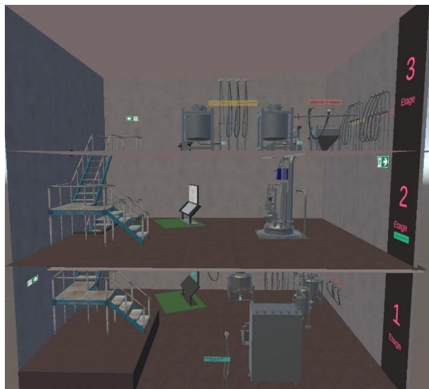
Fig. 2. VR environment of the training prototype for the production of butyllithium (scaled side view) in a 3-level chemical plant. Participants experience the environment in natural scales using an HMD.
