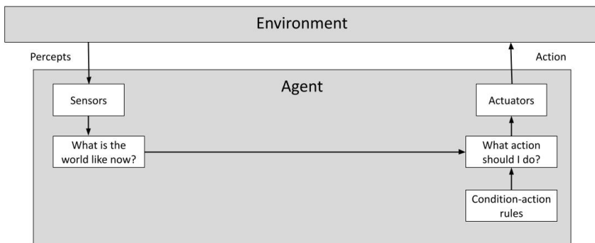
FIGURE 2.2: The typical model of a simple reflex agent, taken from [RN10, p. 49]
