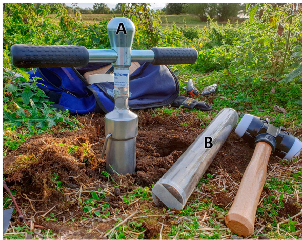
Figure 2. Extraction of undisturbed soil cores at Langmere, Norfolk, UK: (A) the Eijkelkamp 04.17.01.C split tube sampler, and (B) an extracted soil core encased within plastic tubing (9 October 2019). Photograph: D. A. Callaghan.
