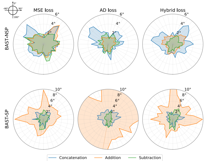
Figure 2: The angular distance (AD) error of the proposed BAST in each azimuth with different loss functions and interaural integration methods.
