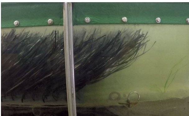
Figure 1. Utilized artificial seagrass (ASG) made out of a PVC plate and 30 cm long PP-ribbon stripes and one transplanted seagrass shoot in the flume.
