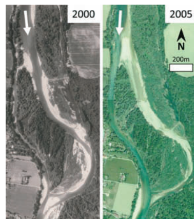
Figure 3. The evolution of a two channel system near Mollon (Case A) where the main channel switches due to a difference in channel slope. (IGN-France and Google earth).
