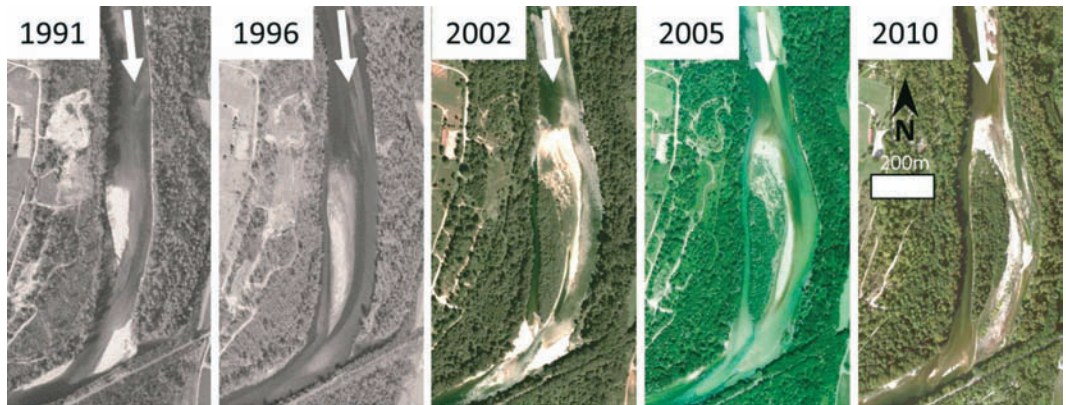
Figure 6. Formation of a bar in the main channel upstream of Pont de Chazey (Case D) which divides the flow in two channels. (IGN-France, Google Earth and Esri).
