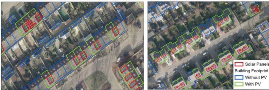
Figure 2-10: Results of the post-processing steps to compensate for FP's, missing panels and to assign panels to the right building with Orthos.
