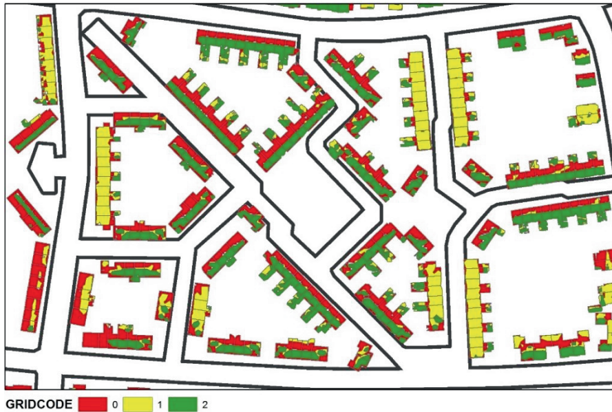
Figure 3-6: Final output showing the geographic potential. Grid code 0 shows unfeasible areas, 1 represents partially suitable area and 2 shows best suits areas for the deployment of PV
