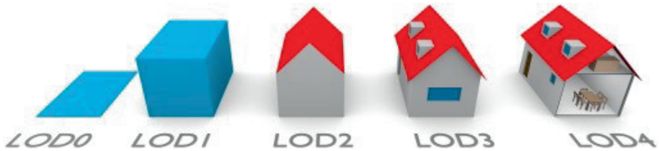
Figure 8-3: explanation of 3D models available at different level of detail. Source: [264]
