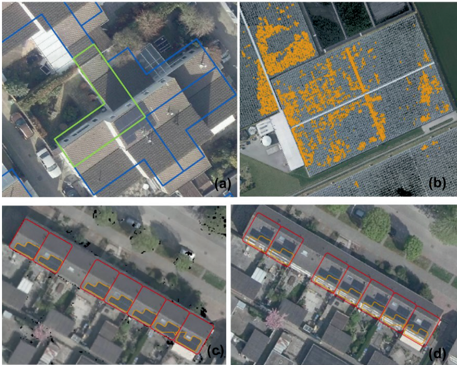
Figure 2-6: (a) Displacement problems causing confusion in panel assignment to a building, solved using post-processing. In this case the panel has been assigned to the building represented in green, (b) identified false positives on green houses, (c) panels detected from TOs and (d) panels detected from Orthos.
