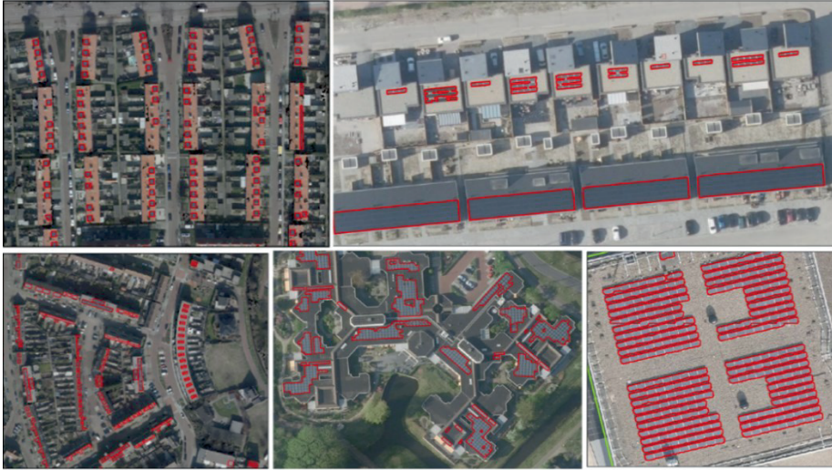
Figure 2-8: Results of the DL algorithms on different building types. Solar panels have been detected with location and shape accuracy. These results are the combination of two modes variants described in Section 2.4.1.
