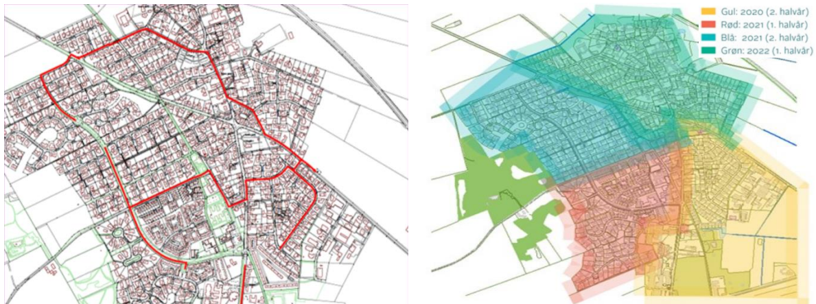
Figure 3. Map of the planning of the main pipeline for Strovorde (left) and zones for the intermediate pipes and its respective estimated time of construction (right) (Aalborg Forsyning, 2021b)
