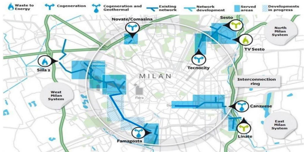
Figure 9. Map of the existing network infrastructure and planned expansion of the district heating network in Milan (Heat Roadmap Europe, 2017)
